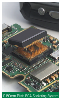
0.50mm Pitch BGA Socketing System
